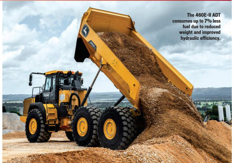
The 460E-II ADT consumes up to 7% less fuel due to reduced weight and improved hydraulic efficiency.
