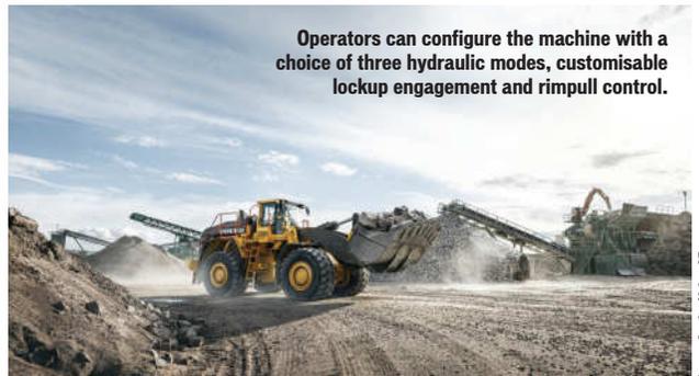
Operators can configure the machine with a choice of three hydraulic modes, customisable lockup engagement and rimpull control.
