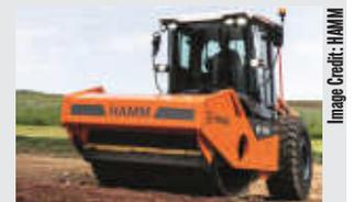
**With operating weight of 11-25 t and a wide range of equipment variants, the HC Series can comply with a wide range of requirements.**
