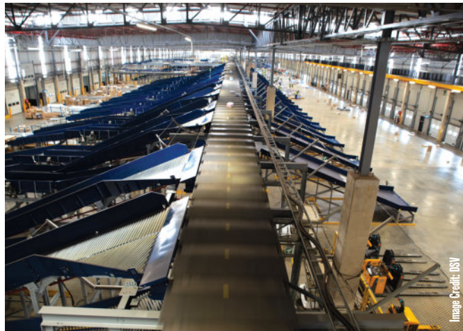
The cross-dock sorter can handle 13,000 packages every hour.
