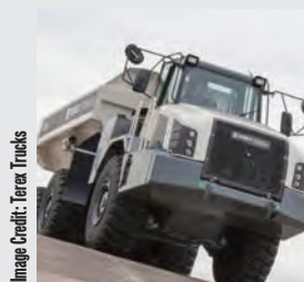
The TA300 articulated hauler has a new transmission, improving efficiency.
