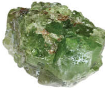
CO 2 will be stored in olivine, which will then be used to make green cement.
