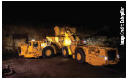
The loader's redesigned buckets are available in four sizes to match material density needs.
