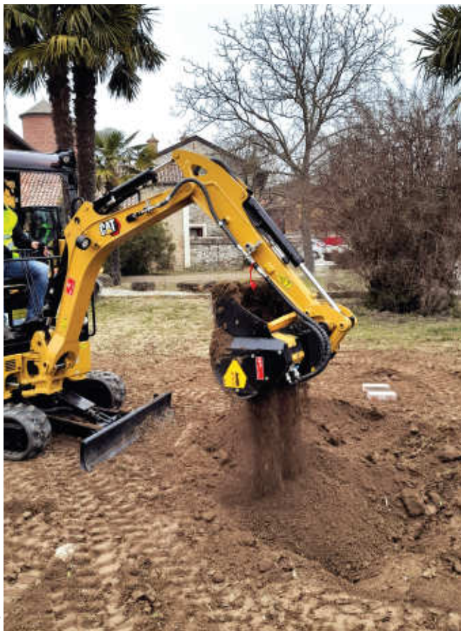
The MB-HDS207 is compatible with a mini excavator with operating weight from 1.3 to 2.8 tons.
