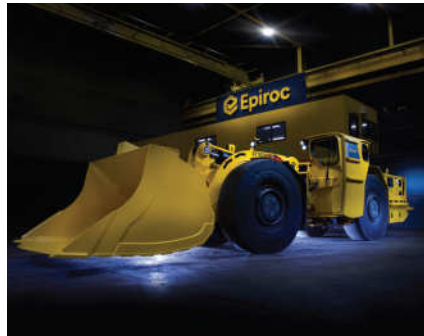
An Epiroc Scooptram ST1030 loader that has been converted from diesel to battery electric.
