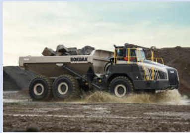
The 38 tonne RA40 is powered by a Scania DC13 engine.
