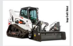
The Heavy Duty Box Blade is suitable for use with most of the models in the Bobcat skid-steer and compact track loader ranges.
