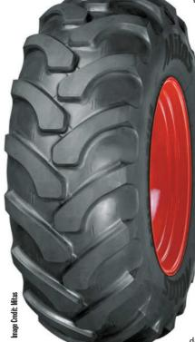
The new GRIP'N'RIDE construction tyre is larger than the existing 19.5L - 24 IND tyre.
