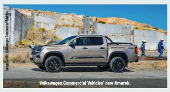
than its predecessor and its wheelbase of 3,270 mm represents an increase of 173 mm to provide more room. Four turbo diesel (TDI) engines and one turbocharged petrol engine have been developed for the new Amarok to provide efficiency and high levels of torque. On the African market it is the base specification engine that is being used: a four-cylinder, 2.0 litre TDI delivering 110 kW.
