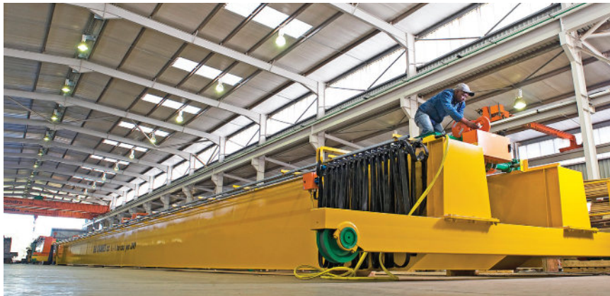
Very wide-span double girder overhead crane nearing completion in Condra's Johannesburg factory. The two 40-ton cranes for Paragon Steel Structures, which will each have a span of 28 metres, are similar to the crane in this photograph.
