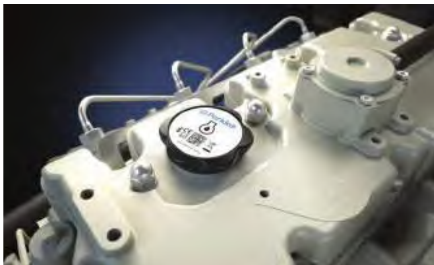
The Perkins Smartcap monitors Perkins engines and sends data direct to the Perkins My Engine App. (Source: Perkins)
