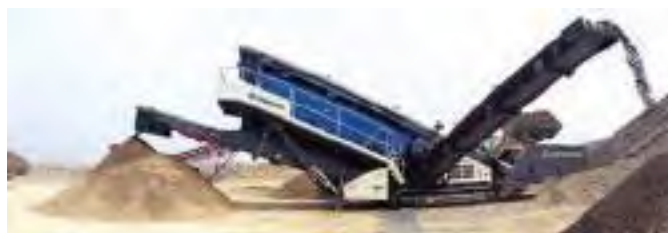
The new Kleemann MS 953 EVO classifying screen is suitable for nomadic crushing contractors. (Source: Wirtgen Group)
