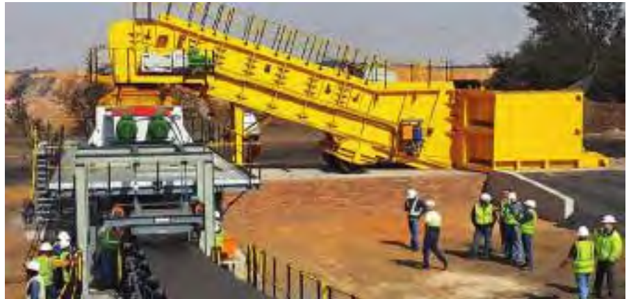
PC Kruger, capital sales manager at FLSmidth Buffalo, said feeder breakers are well suited for most underground mining operations where the coal is relatively soft. (Source: FLSmidth).
