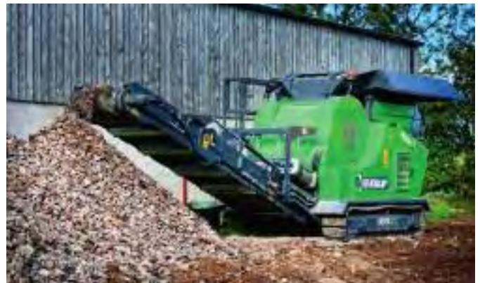
The Bison 120 jaw crusher features a 680mm x 400mm single toggle jaw crusher. (Source: EvoQuip)
