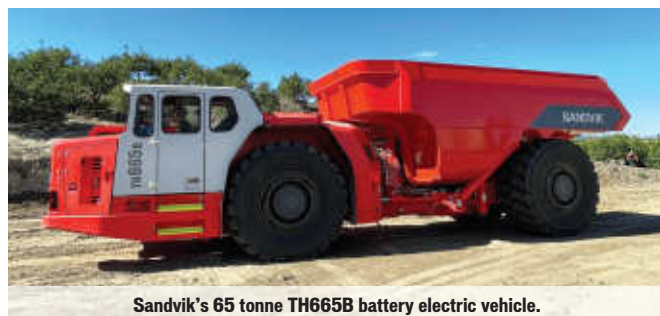
Sandvik’s 65 tonne TH665B battery electric vehicle.
