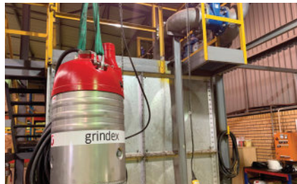
The Grindex Bravo being hoisted into Integrated Pump Technology's in-house test sump.
