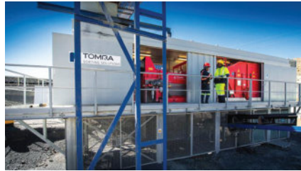
The technology recognises and separates material based on its specific atomic density.
