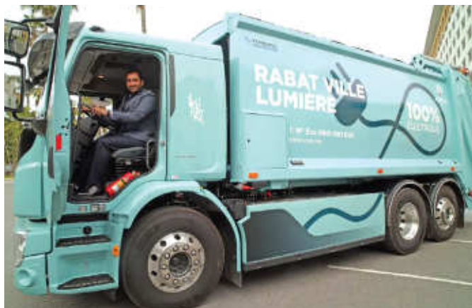
A series-produced, zero-exhaust emission truck will be used for collecting waste by the company Arma in Rabat.
