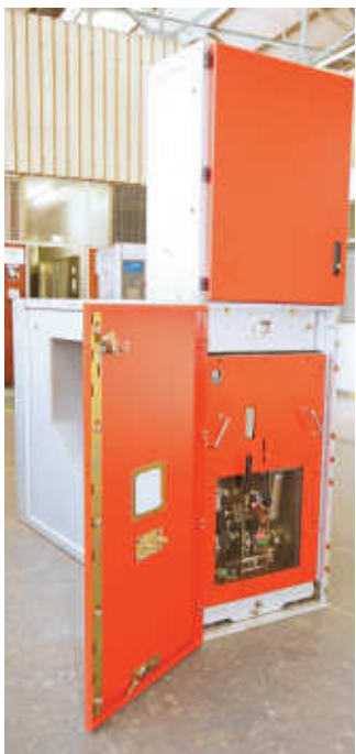
SBV4XE switchgear panels being assembled in ACTOM MV Switchgear's factory.
