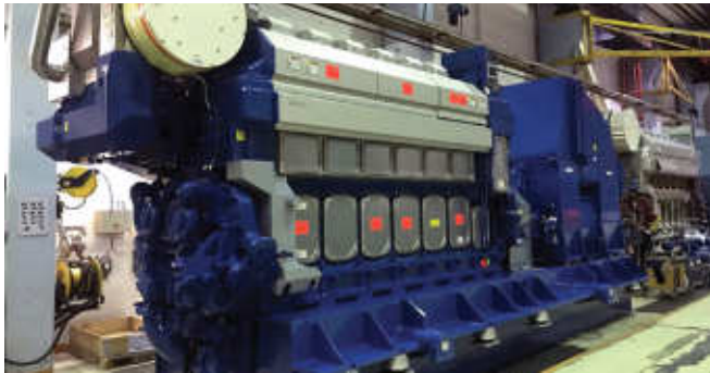
The Wärtsilä 32 engine, six of which are being used in the Benguela Gem vessel.
