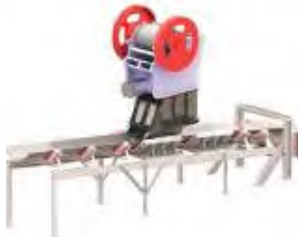
A typical transfer point discharging onto a conveyor.
