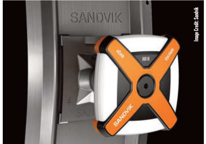
The retrofitable design of xCell Cyclops sensors makes them very easy to install directly onto existing rock bolts.
