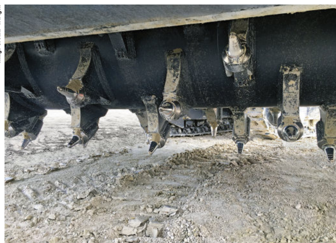
Wirtgen's powerful milling drums can produce significantly smaller grain sizes than, for example, drilling and blasting or, as shown here, using a dozer.
