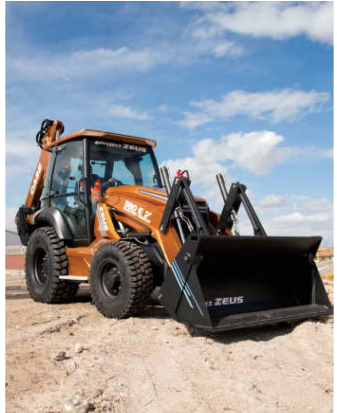
Case Construction unveiled the 580 EV, fully-electric backhoe loader at the end of 2020.
