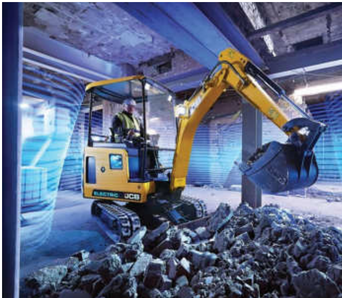
In 2019, JCB launched its first-ever fully-electric mini excavator, the 19C-1E.
