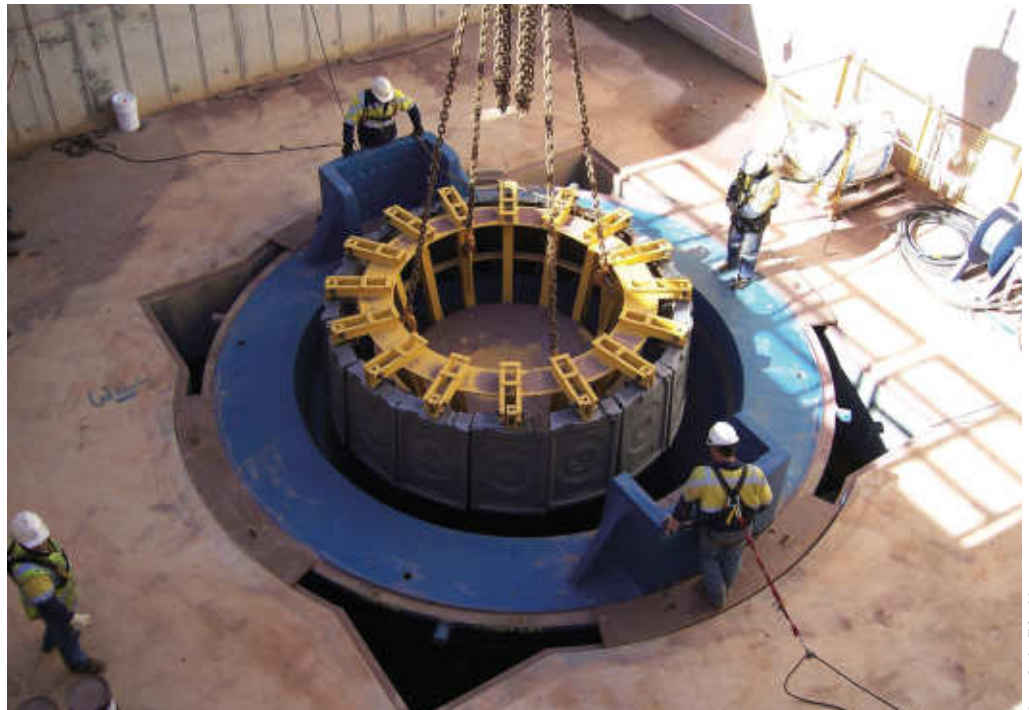
With FLSmidth’s top service range of gyratory crusher models, 95% of the servicing can be conducted from the top.
