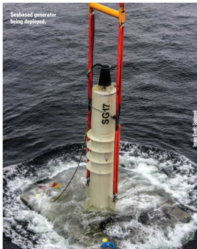
Seabased wave power parks produce electricity by absorbing and transforming the kinetic energy of the ocean waves into electrical energy suitable for grid use.
