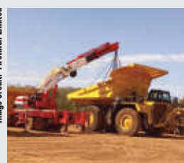
New Komatsu 785 haul truck being assembled onsite at Morila.
