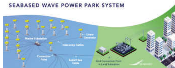
Seabased wave power parks produce electricity by absorbing and transforming the kinetic energy of the ocean waves into electrical energy suitable for grid use.
