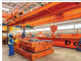
The 30/10-ton maintenance crane being prepared for load test, showing digital readouts (left of photo) and the underslung auxiliary hoist in the background.
