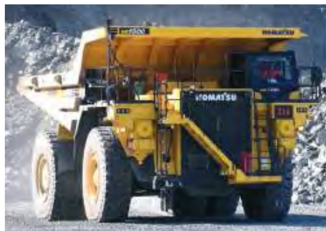
Komatsu's HD1500-8 is powered by a 50-litre engine.
