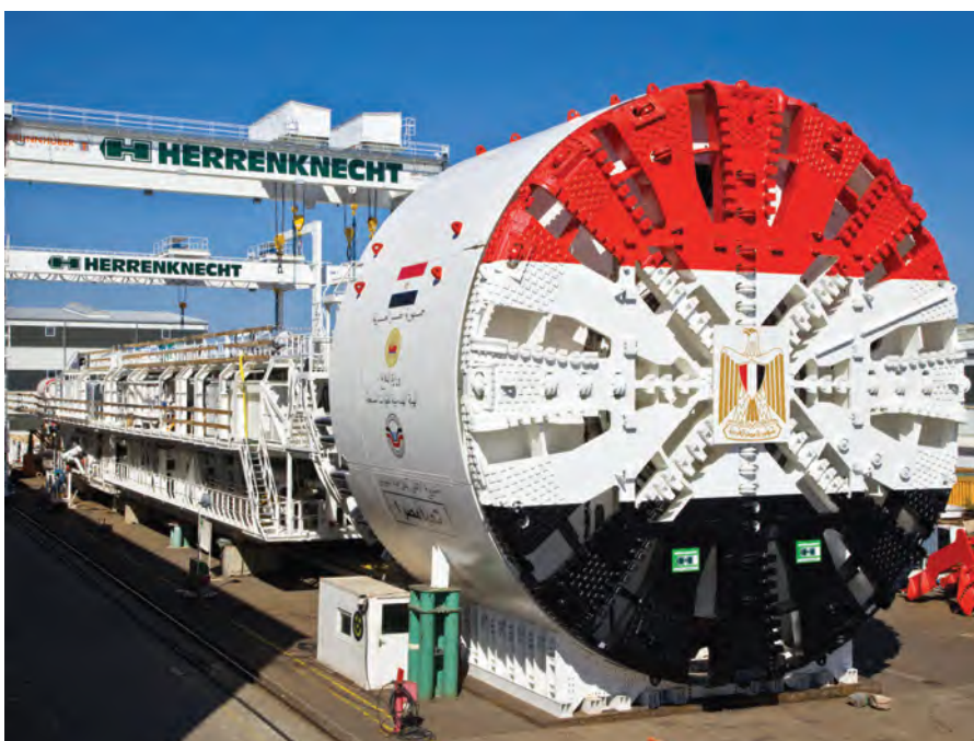
Four tunnel boring machines were supplied by Herrenknecht for the construction of two new road tunnels under the Suez Canal.
