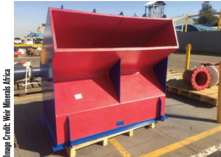
Image Credit: Weir Minerals Africa Linatex premium rubber and Linard 60 rubber combination installed on a typical chute.
