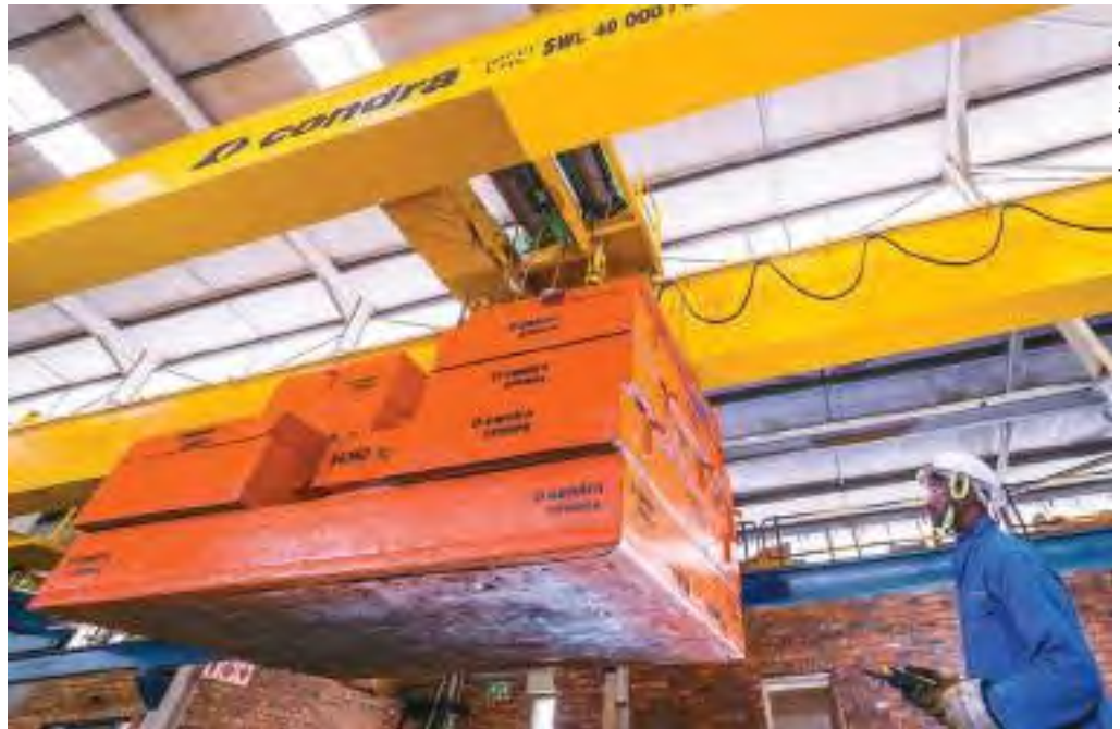
A Condra double-girder electric overhead travelling crane undergoing testing at the company’s Johannesburg factory.
