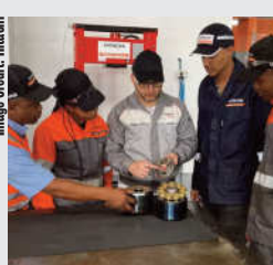
Remanufacturing a main pump.
