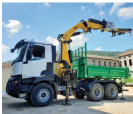
The cranes have from two to eight extensions.
