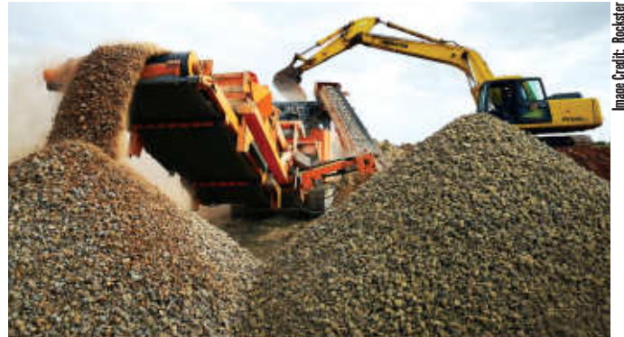
The final product produced by the Rockster R1100D is well shaped cubic grain of high quality, as was certified by laboratory.
