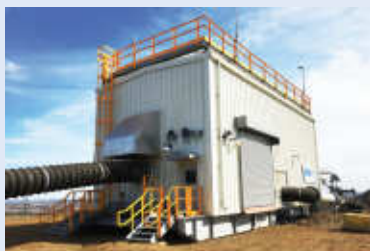
The Weir pumphouse can be used for mine dewatering and slurry transportation.
