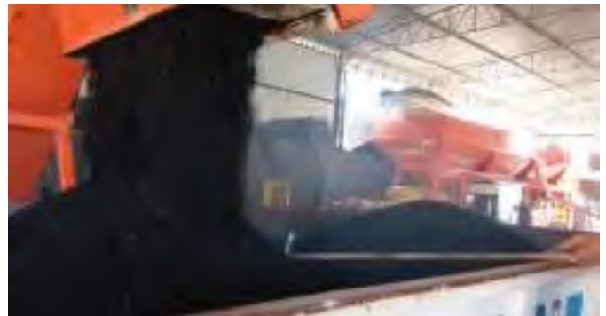
Discharge bin with geometry to avoid heterogeneous mix. (Source: CIBER)
