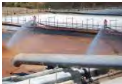
Integrated Pump Rental's Slurry Blaster hydro mining equipment solution was deemed the most appropriate for this harsh application at a copper mine in the DRC
