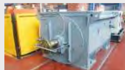
Marthinusen & Coutts recently completed the rebuild of a 6 550kW two pole 11,000 Volt squirrel cage induction blower motor for a copper mine in Zambia
