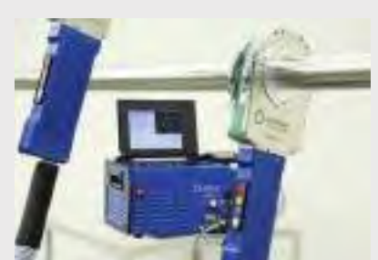
The Orbimat 165 CA power supply for orbital welding
