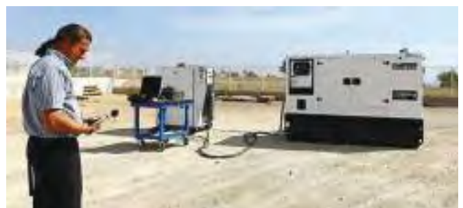
A noise emission test on the IIRN-165 unit (Source: Inmesol)
