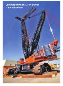
referred to as the load moment. Most hydraulic cranes are rated at their capacity at 3 metres, whereas the rating for a lattice boom crane is based on a larger load moment, which can be anywhere between 7 and 14 metres, with this capacity based on its structural integrity. In essence, a lattice boom crawler crane is capable of performing far heavier lifts and offers greater flexibility in terms of its application because of its pick and carry capability," he said.
