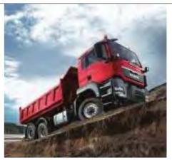
MAN HydroDrive is the only all-wheel system that can get traction on to the front axle of a normal and medium-height truck
