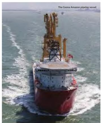
designed to operate in tandem to support work in water depths of up to 3,000m (10,000 ft), enable her to easily install large manifolds and heavy subsea structures. This combined with the vertical-lay pipelay system featuring a top tension of 600te, capable of laying rigid pipe to 3,000m (10,000 ft) water depth make her a vessel of choice for all deepwater field development needs.
