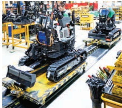
E10e assembly line at Bobcat's compact equipment manufacturing plant at Dobris, in the Czech Republic.
