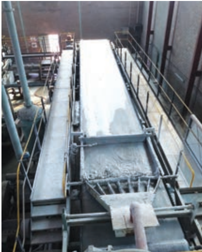
One of two conveyor belts for the first stage of moisture removal from gypsum slurry before it leaves the washing plant at OMV's Potchefstroom facility.
