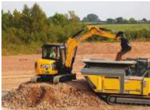
The 65R-1 features an H-frame undercarriage and a choice of tracks for strength, durability, and flexibility
