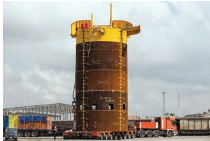
The 16 modular axle-lines from Faymonville were used in the transportation of the huge suction pile.
