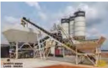
The Elkon Mobile Master-135 Jaguar Mobile Concrete Batching Plant
