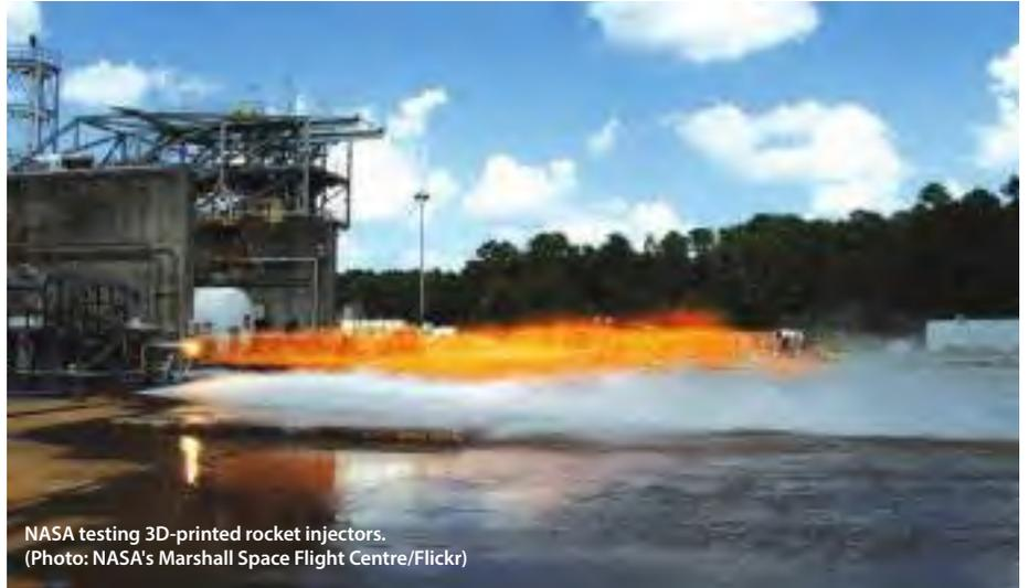
NASA testing 3D-printed rocket injectors.
