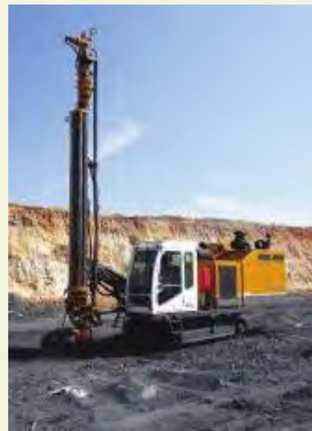
Hausherr HSB 3000 blast borehole drilling rig in Kazakhstan
