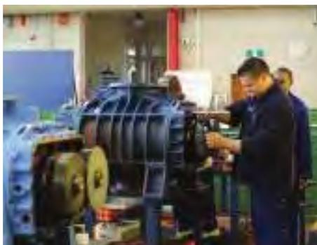
A blower being overhauled in an Aerzen Airgas servicing area
