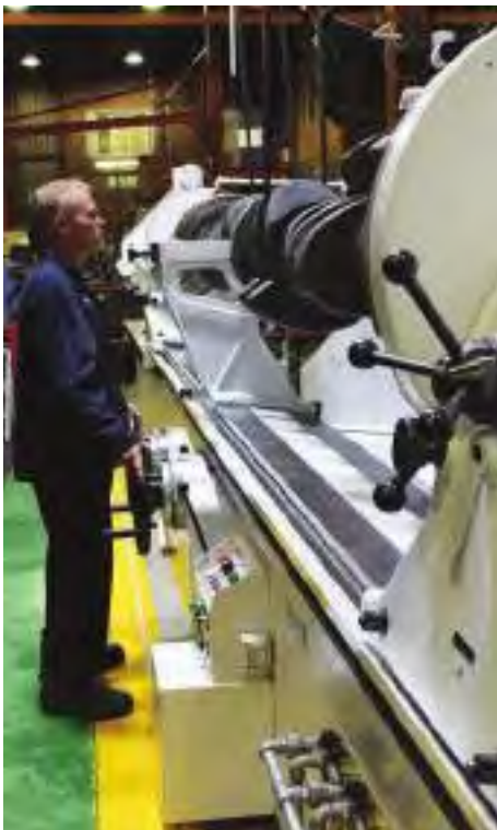
The enormous crankshaft grinder at Metric Automotive Engineering can easily handle shafts of up to 4.7 metres long with weights of up to five tons
