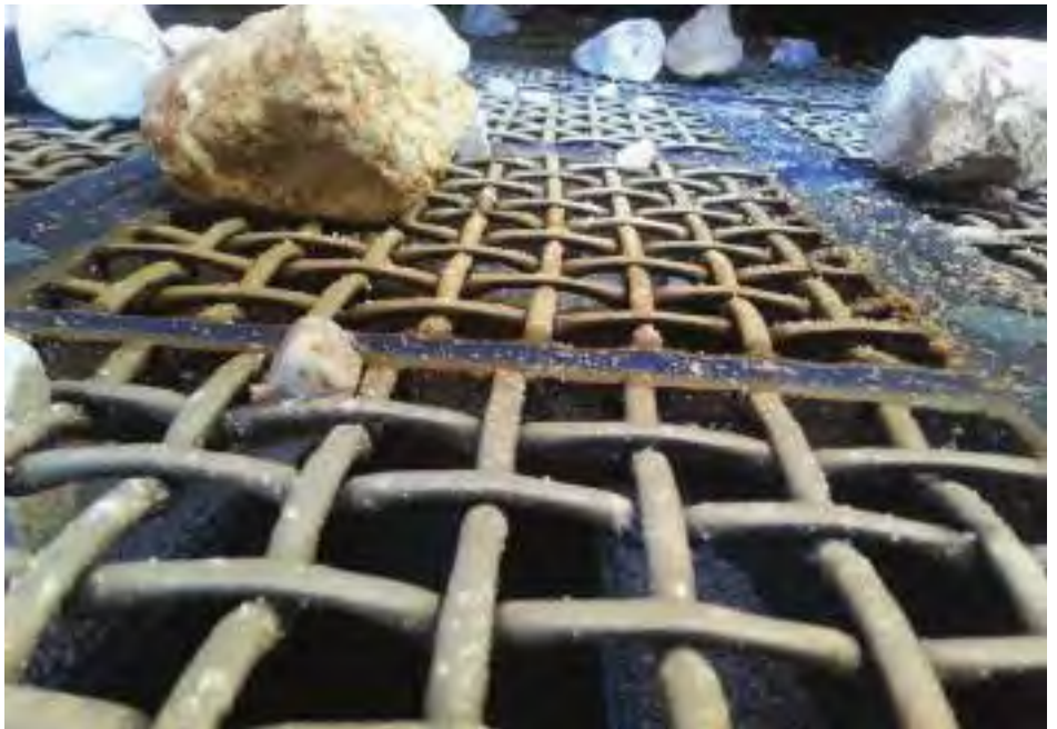
FLSmidth has designed a hybrid poly wire modular panel for use in Rietvlei Silica Mine's screening process
