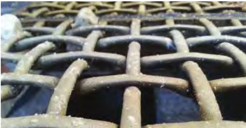
FLSmidth's hybrid poly wire modular panel is a standard 1'x1' panel comprising a flat top woven wire screen
