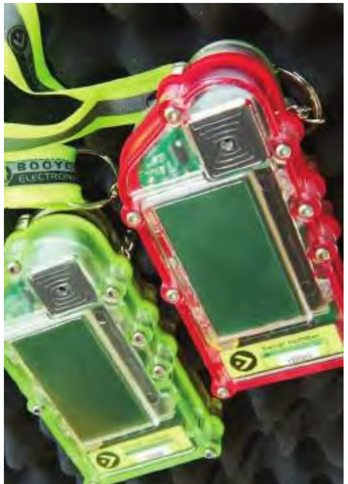
The Sentient handheld gas detection device is a multi-gas instrument, which measures relative humidity as a standard offering
