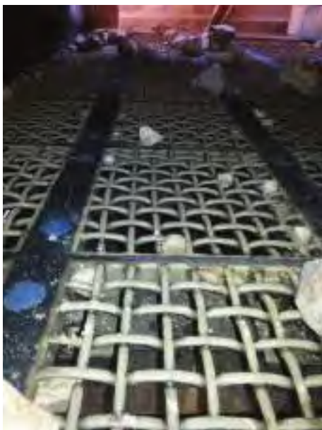
FLSmidth's hybrid poly wire modular panel
