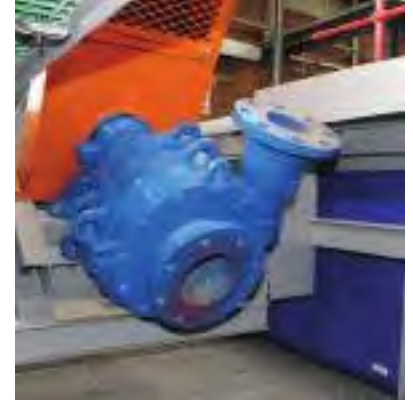
One of two Warman DWU 125 dewatering pumps mounted to a pontoon and walkway during assembly phase
