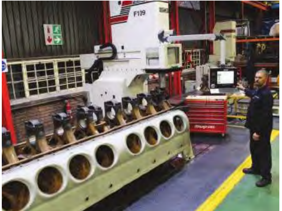
The new CNC machining centre, which has added capacity for Metric Automotive Engineering to handle the huge engine blocks found in the marine sector
