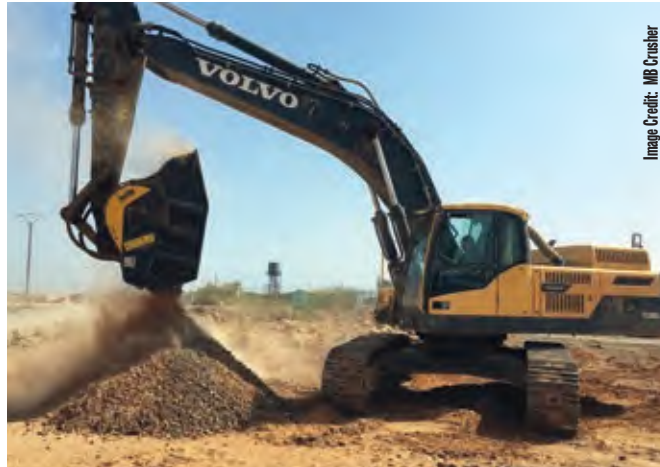
The MB Crusher Bucket BF120.4 in action at the Djibouti International Free Trade Zone. It can crush more than one million cubic metres of basalt for road construction purposes.
