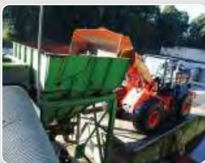
The ZW220HYB5 is easy to operate; using travel motors rather than the conventional transmission, there are no jolts when digging or climbing uphill
