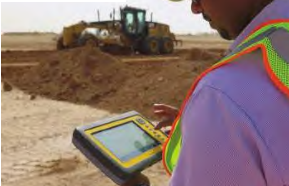
Cat Grade Control allows machine operators to achieve greater grading accuracy (Photo: Cat)
