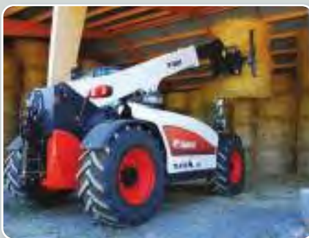
The TL470HF telescopic handler offers higher horsepower engine and a 190l/min load sensing hydraulic pump
