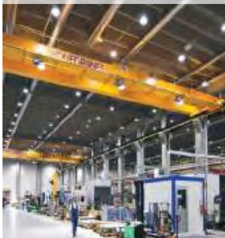
CXT Wire Rope Hoist crane equipped with many of our Smart Features, like ESR (Extended Speed Range) and positioning features; the crane contributes to the speed and precision of ATA's production in Finland
