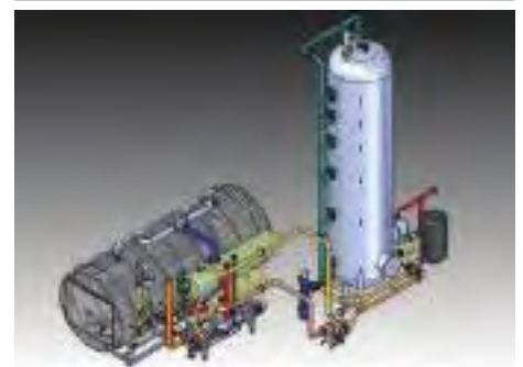
The self-contained, independent system consists of a multilayer storage tank, which is divided into several temperature zones and firmly piped to the steriliser via a heat exchanger
