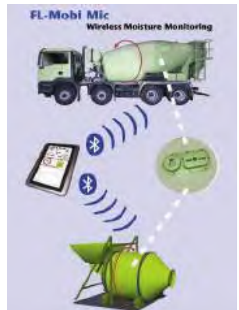
The FL-MOBI-MIC Inspector utilises Bluetooth and GSM technology
