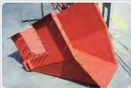
CrC can affect the quality, consistency, integrity and wear properties of long life liner plates
