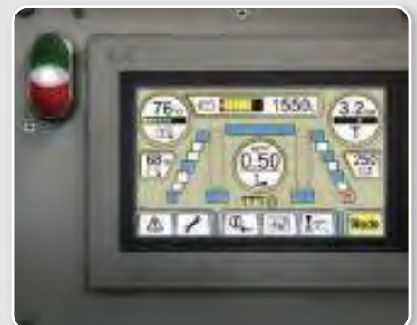
All the settings required for replenishing, circulating and heating the emulsion can be entered and monitored directly via the touchscreen
