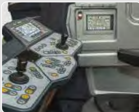
One feature of fundamental importance is that operation of the spray module has been integrated into the ErgoPlus 3 operating concept
