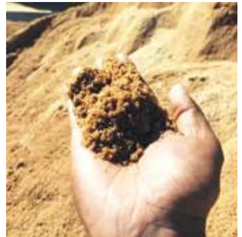
Quality manufactured sands made of washed aggregates are fast becoming the alternative of choice to natural sand
