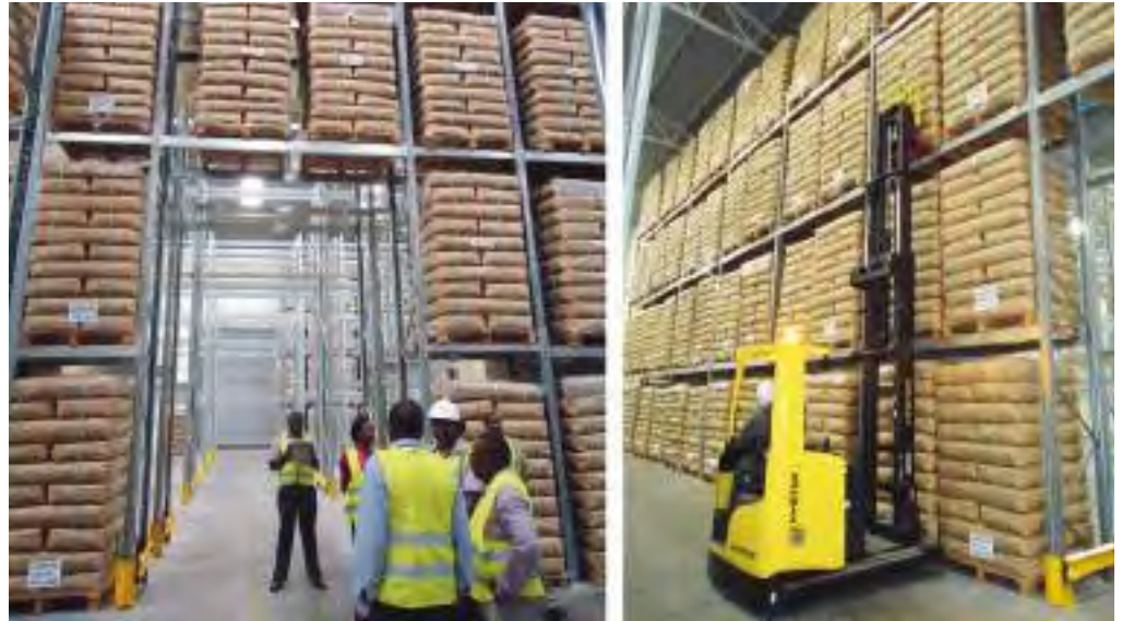
There is now four-level storage, with bridge beams and rack protection barriers
