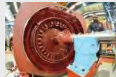
Alpheus Mtshali, from Marthinusen & Coutts, is pictured with the 1,586kW, 187.5rpm, 3,300V, 278 A stator
